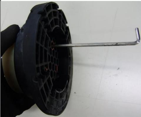
*Screw the standard end stops with the new end stop adapters using the supplied Allen screws (M6x16mm)*
