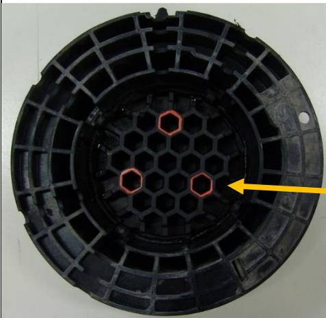
*The standard end stops are to be drilled through on the rear side according to the thread in the supplied end stop adapter.*
